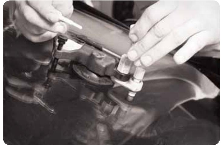
Most rock-chip repairs take 30 minutes or less.
